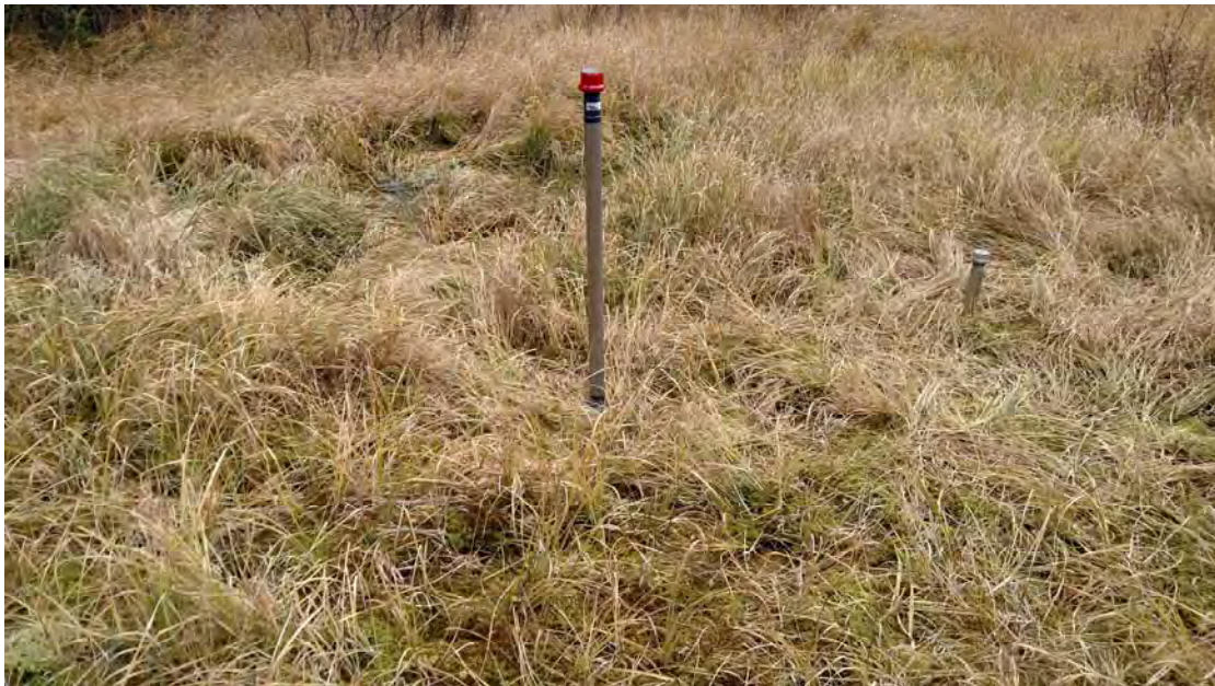
Well FB2 pre-installation (only the point, ~ 3", is in the ground) and post-installation of well FB1 (short well) looking southeast (no pre-installation of FB1).
