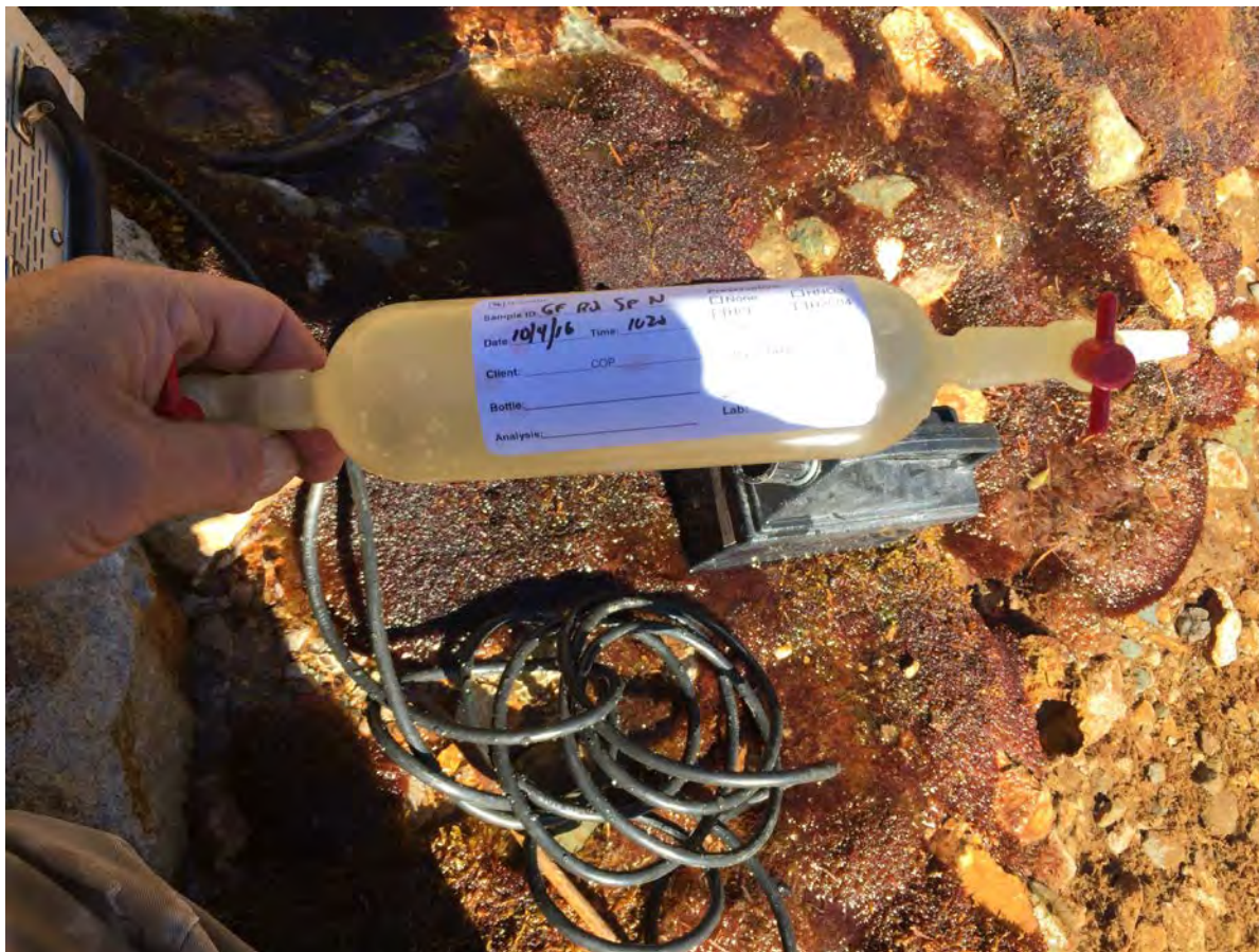
Photo 2. Double ended stopcock cylinder used to collect C14 samples.
