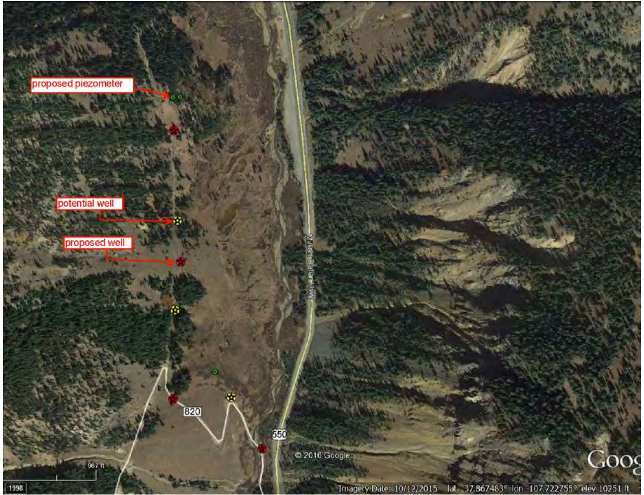
Figure 2. Chattanooga Fen proposed piezometer and well locations.
