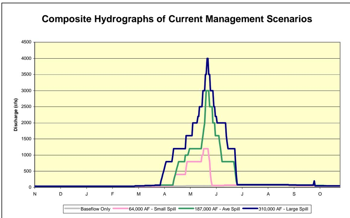
Figure 19. Composite Hydrographs for the four current management scenarios being discussed in this section. The small spike October 1 is the 12-hour, 400 cfs release for fish stocking between McPhee Dam and Bradfield Bridge.
