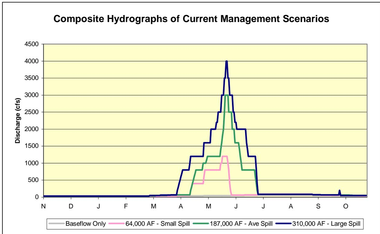
Figure 2. Composite Hydrographs for the four current management scenarios being discussed in this section. The small spike October 1 is the 12-hour, 400 cfs release for fish stocking between McPhee Dam and Bradfield Bridge.
