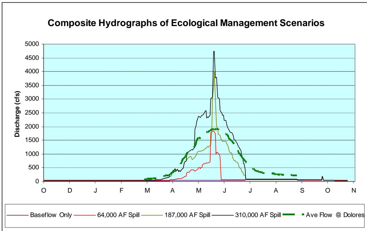
Figure20. Composite Hydrographs for the four ecological flow management scenarios being discussed in this section. The small spike October 1 is the 12-hour, 400 cfs release for fish stocking between McPhee Dam and Bradfield Bridge.
