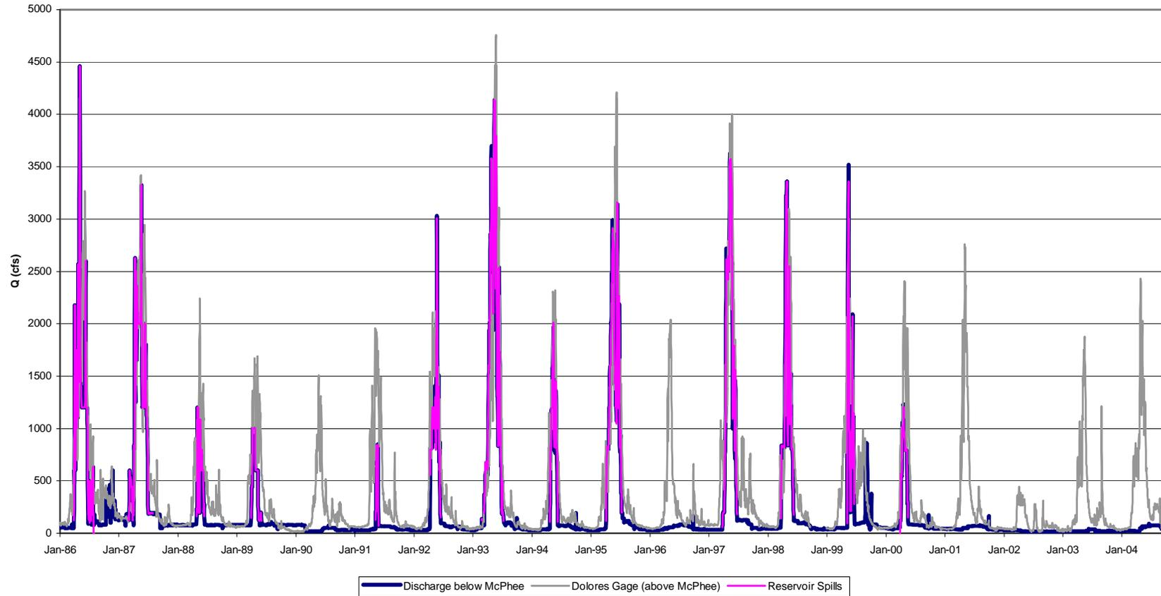
Figure 15. Post-McPhee Hydrology showing gaged inflow at Dolores, and both spill and baseflow releases from McPhee Reservoir.
