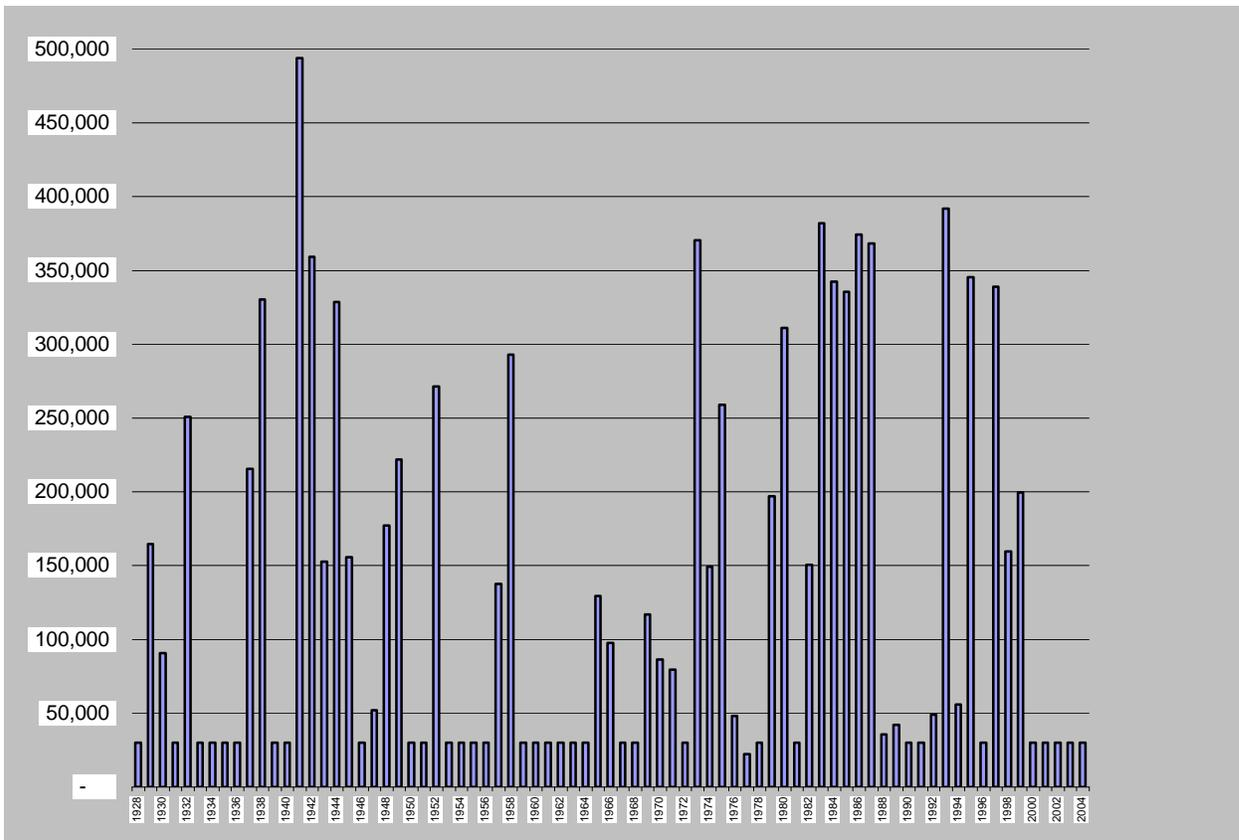
Figure 1. DRD Hydrologic Model output summarized by modeled year. Data includes baseflow (30,000 AF) and one year of modeled shortage in 1977.
