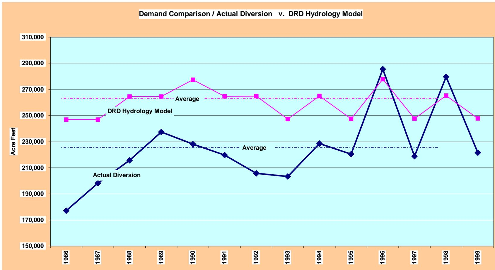
Note: DRD Hydrology model adjusts full allocations of project users by modified usage resulting from wet and dry weather patterns.
