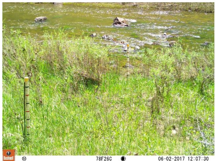
**Figure 4.** Dove Creek staff gage at pre-release, rising water, peak-release, and post-release. Notice river rising substantially out of its banks at peak-release but with very little change in the amount of woody vegetation.
