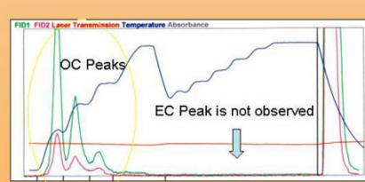
Representative thermogram of our marine site, CSJ. Here, the EC peak is not observed. Only OC concentrations are detected. This clearly show that under our sampling conditions this site was not affected by anthropogenic emissions (EC is a tracer for combustion).
