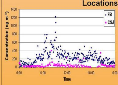
These results show the BC concentrations measured with the aethalometer for a 24-h period. As shown in the previous graph, the highest concentrations (1200 ng m-3) are observed during the hours when the traffic is the highest (6-9am). Daytime concentrations are on average 330 ng m-3 and during the traffic hours 470 ng m<sup>-3</sup>. Nighttime concentrations are on average 130 ng m-3. CSJ average concentrations are 40 ng m-3.
