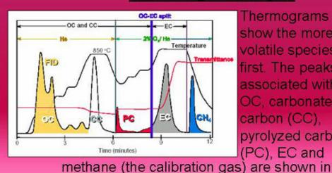
hermograms show the more olatile species irst. The peaks issociated with C. carbonate carbon (CC), pyrolyzed carbon (PC), EC and
