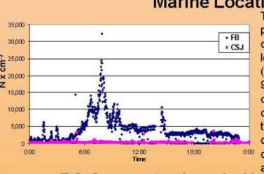
The blue line shows the typical profile for particle number concentrations (24 h) at our urban location. The highest concentrations (33000 cm-3) are observed around 6-9am (high traffic). Daytime concentrations are on average 5500 cm<sup>-3</sup> and 10400 cm<sup>-3</sup> during the traffic hours. Nighttime concentrations are on average 2000 cm<sup>-3</sup>. CSJ average concentrations are 370 cm-3
