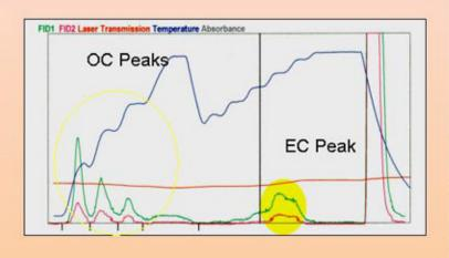
Typical thermogram of an urban site, in this case, FB. Defined by the green line, two areas are highlighted. At the beginning (left side of the graph), three distinctive peaks (most volatile ones) are observed. These represent the concentration of OC in the filter. The other area is composed of a broad peak. This is a typical signal for EC concentration.
