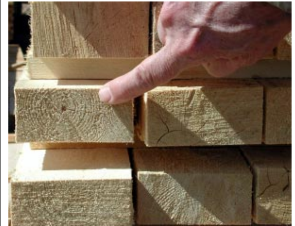
“Small diameter is not always poor quality, or unusable, or for chipping only,” said Randy Roper, pointing out a stack of freshly sawn lumber, to be used for fencing or some other non-structural building project. Note the rings depicting the center of the small log from which the 2x4s were sawn.
