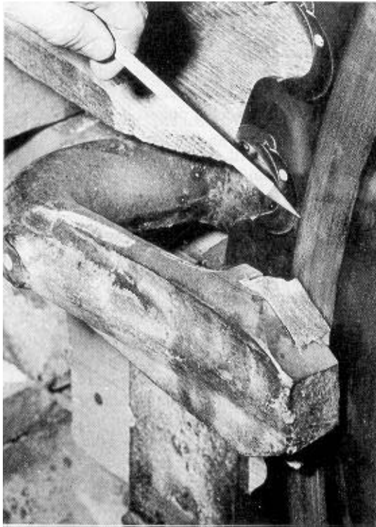
Figure 24. – The wear mark on the saw denotes the position of the guide pins. Pins should not make contact with the base of the shanks.
