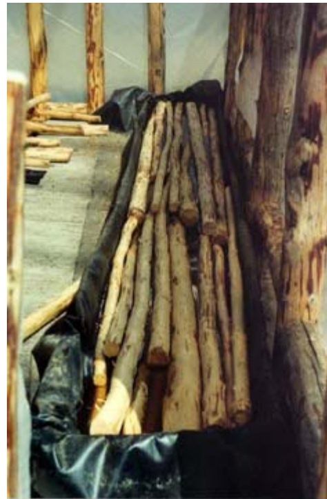
Project members hope that green logs soak in a borate-based dip will provide an alternative niche product to toxic preservations used in the US.
