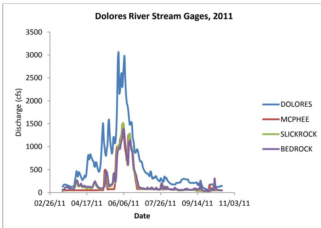
**Figure 7.** Dolores River hydrographs for water year 2011, with discharge data from four gauging stations superimposed to show matching of peak discharge above and below McPhee Dam. Gages are listed, from top to bottom, in upstream to downstream order: Dolores at Dolores (above dam, unregulated), Dolores below McPhee Dam, Slickrock gage (upstream of Big Gypsum Valley) and Bedrock gage (downstream of Big Gypsum).
