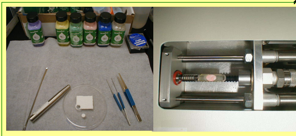
Figure 3. Shows temperature indicating products (TEMPILAQ) plus quartz filter punch plus a Tempilaq sample loaded in the carbon analyzer instrument.
