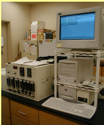
Figure 1. Shows one DRI Model 2001 #6 Thermal/Optical Carbon Analyzer and what is inside of each instrument.
