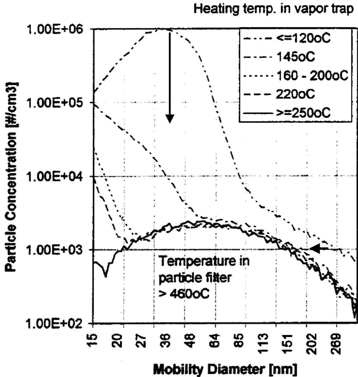
Figure 4. Solid particles and spontaneous condensate in diluted exhaust gas at different temperatures of a thermodesorber (Mayer et al., 1998).
