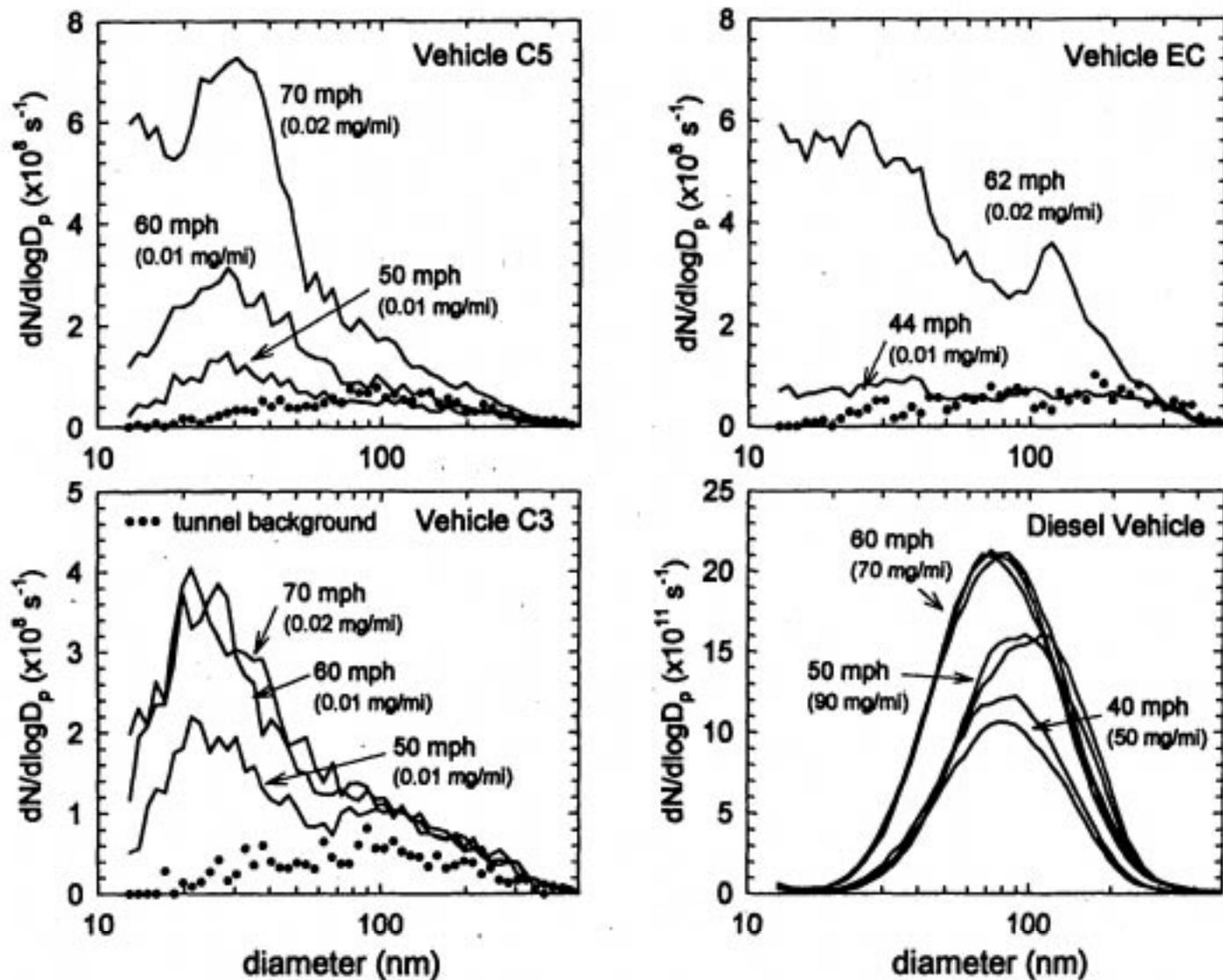
Figure 1. Dependence of particle emissions on vehicle speed for three gasoline cars and one diesel car. Dilution air particle size distributions are given as dotted lines. Exhaust flows for vehicle C5 are 0.010, 0.014, and 0.020  $\text{m}^3/\text{s}$  at 50, 60, and 70 mph. For vehicle C3 they are 0.014, 0.019, and 0.026  $\text{m}^3/\text{s}$  (Maricq et al., 1999).
